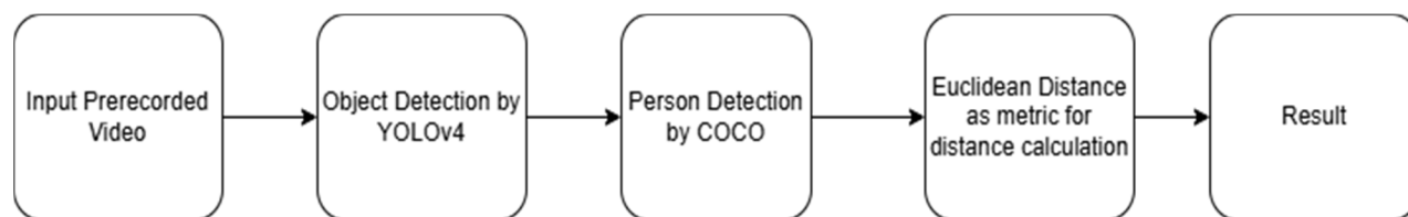
Fig. 3.1 System Architecture of face mask and social distancing
