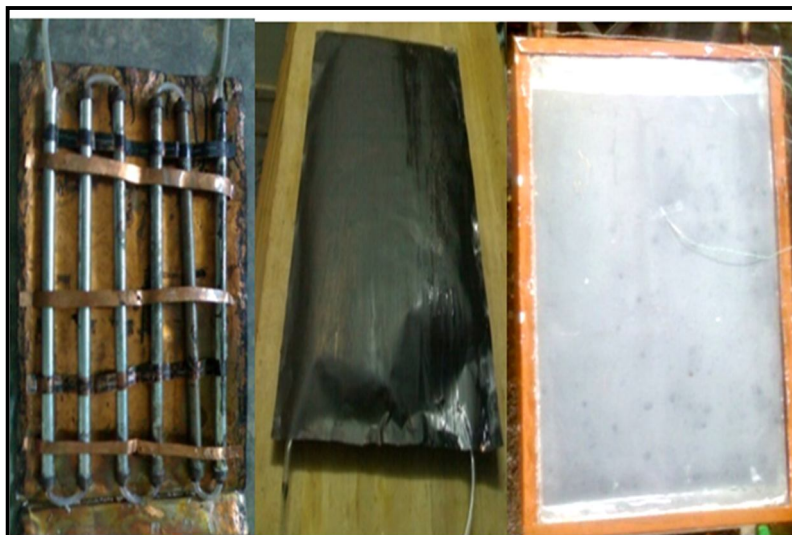
Fig. 4: Copper Foil Sheets with Iron Pipe Filling PCM and Glass Covered
