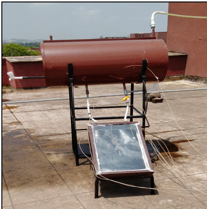
Fig. 5: Experimental set up of flat plate collector
