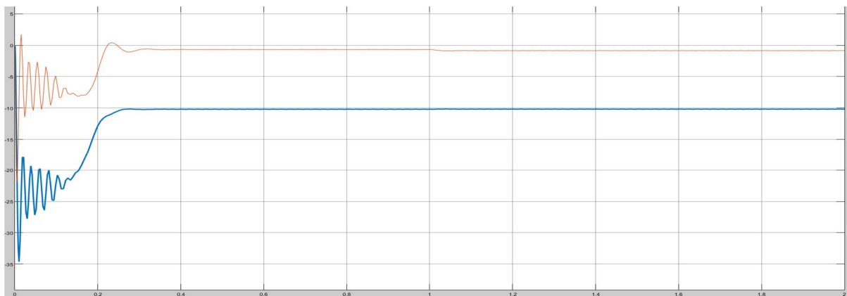
Fig. 11. Current waveform of stator in d-q frame without considering end effects
