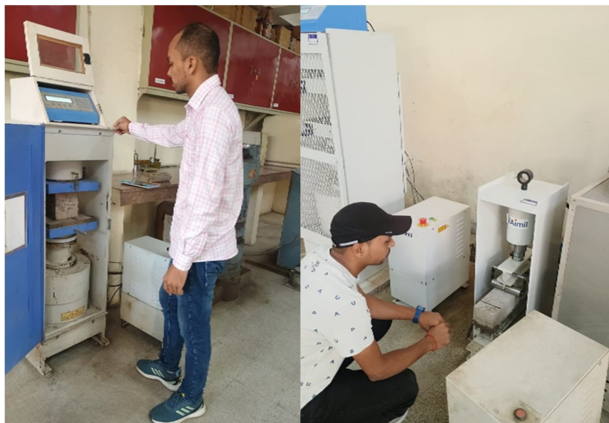
Fig.3 Compressive & Flexural strength test
