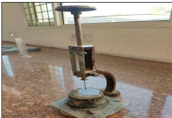
Fig.1 Initial setting time experiment on Vicat's Apparatus
