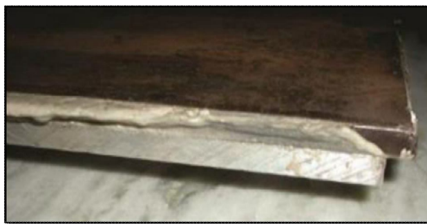
Fig. 2 Carbon Steel/Epoxy/Aluminium Laminated Metal Composite (LMC)
