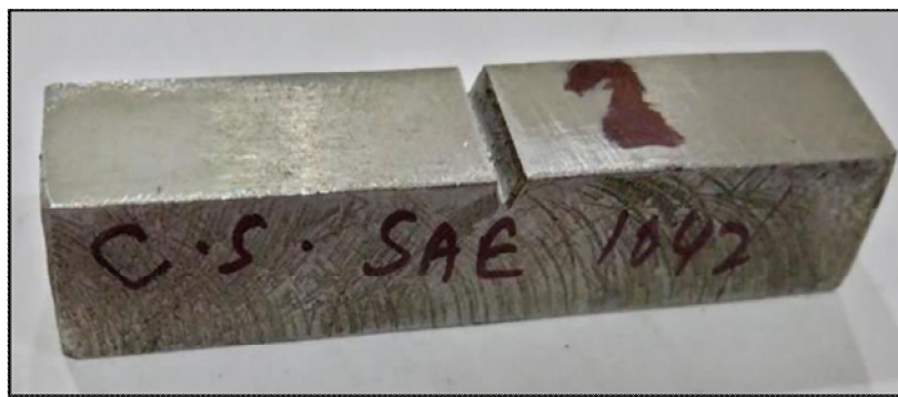
Fig. 7 SAE 1042 Carbon Steel Charpy Test Specimen
