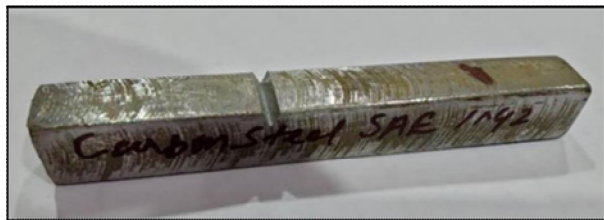
Fig. 3 SAE 1042 Carbon Steel Izod Test Specimen
