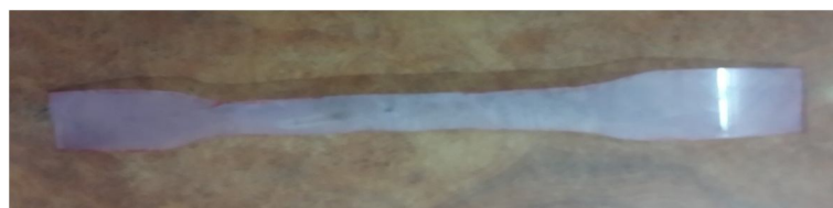
Fig. 6. Specimen wrapping without carbon fibre
