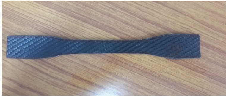
Fig. 7. Specimen wrapping with carbon fibre
