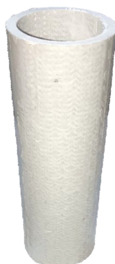
Fig. 1 Pultruded GFRP Round Tube
