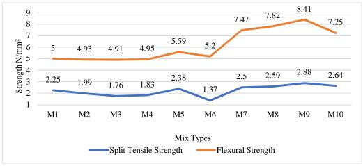
Fig 2: Split Tensile & Flexural Strength of Concrete for 28days
