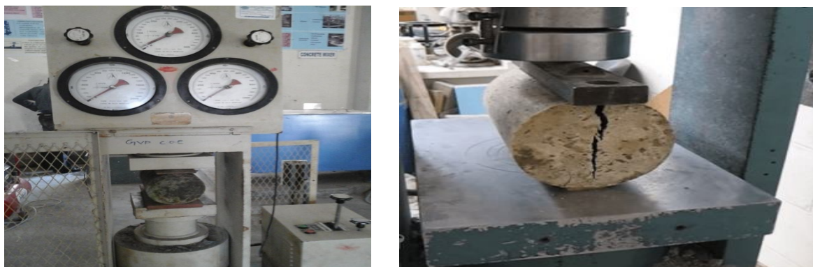
Fig 4.3 testing of specimens for split tensile strength
