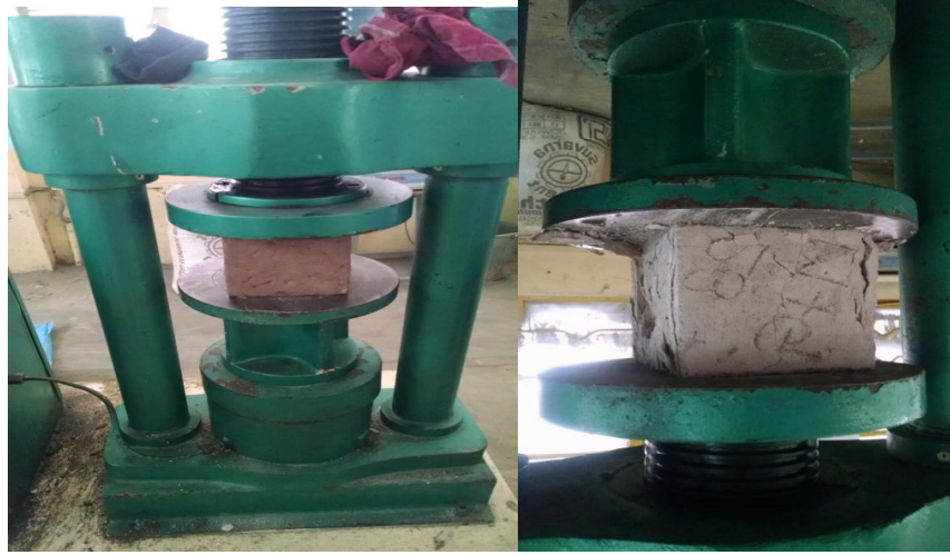
Fig 4.2 – testing of cubes for compressive strength
