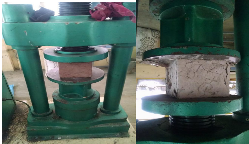
Fig 4.2 – testing of cubes for compressive strength
