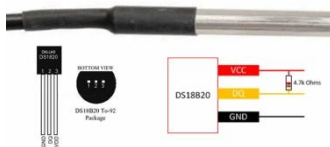
Figure 3. DS18B20 Temperature Sensor
