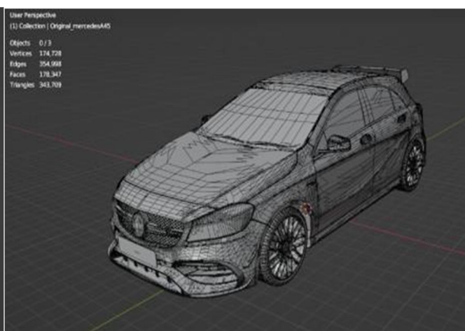
Fig. 11 Angle limit – 1 degree (178,347 faces)
