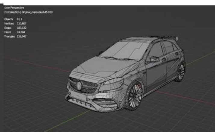
Fig. 15 Angle limit –5 degree (74604 faces)
