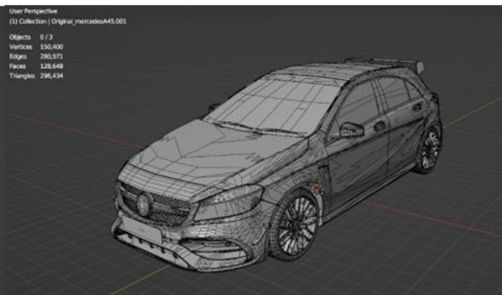
Fig. 13 Angle limit – 2 degree (128648 faces)
