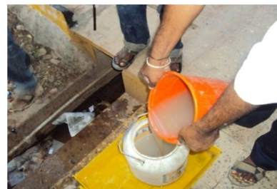
Fig. 3 Mixing of \text{Na}_2\text{SiO}_3 with NaOH
