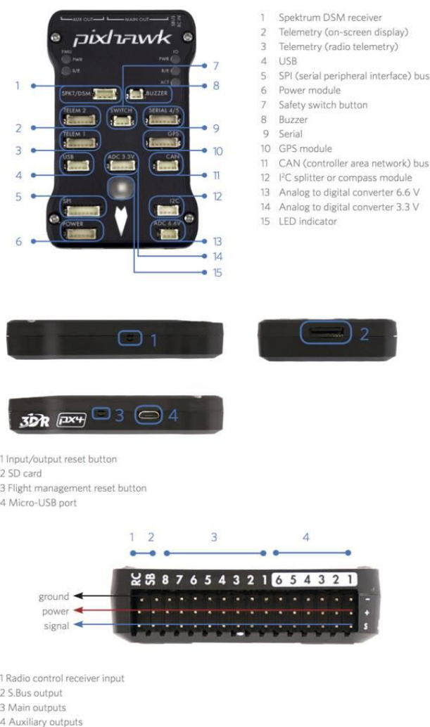
Fig: 6.10 Flight Controller Detailed Picture
