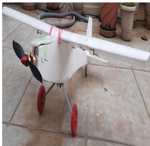
Fig: 7.1 Test Model of Proposed Fixed Wing UAV
