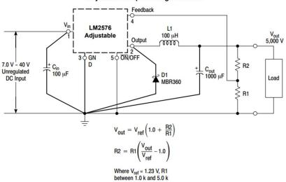
Where the R2 is 10 turn Potentiometer 50KRwhich is controlled by manually, by varying the R2 value we can adjust the output voltage from 1.23 to 37V when R1 needs to be fixed as per calculation. (Ref. No. 2 Onsemi conductor datasheet)
