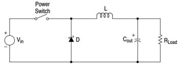
The next period is the "off" period of the power switch. When the power switch turns off, the voltage across the inductor reverses its polarity and is clamped at one diode voltage drop below ground by the catch diode. The current now flows through the catch diode thus maintaining the load current loop. This removes the stored energy from the inductor. The inductor current during this time is.
