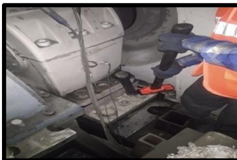
Fig-4: Bump hammering test
