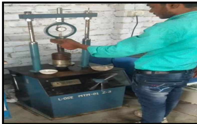
Figure-: Extrusion of mould
