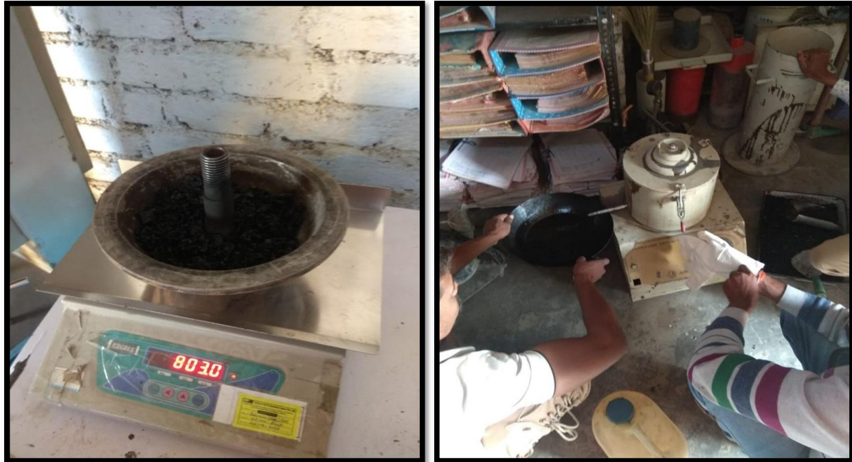
Fig-: Bitumen Extraction test of milling material
