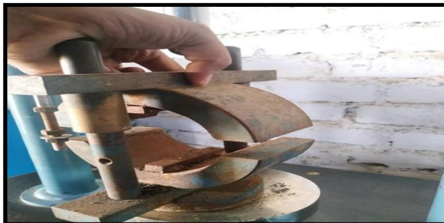
Figure:- Modified version of marshall test apparatus
