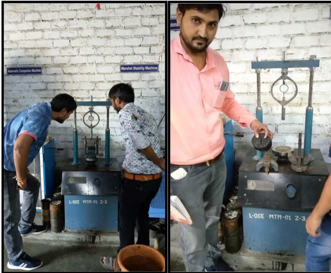
Figure-: ITS Testing in wet condition
