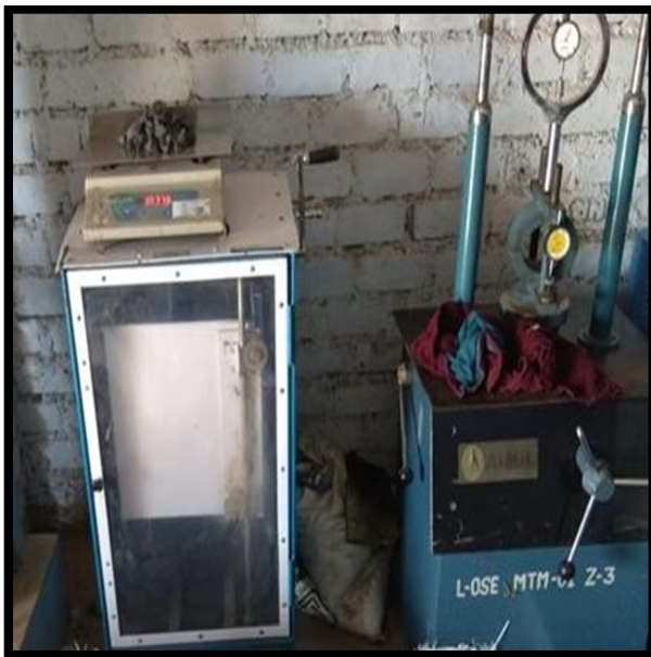
Figure-: Specific gravity and water absorption test on 20 mm down aggregate
