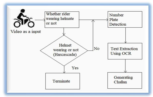
Here we have taken image of the bike racer as an input then it checks whether racer it wearing helmet or not. It checks the helmet wearing or not through the haarcascade algorithm if yes then it terminate the process, and if not then it check the number plate through the text recognition using OCR technique then after the text recognition and number plate detection it generate the chalan receipt and then it debited the money from the bike owner.
