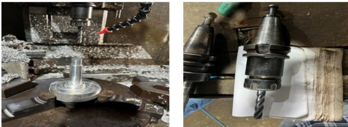
Figure 4 modified component manufactured and Tool bit used for process in CNC using Al 6061
