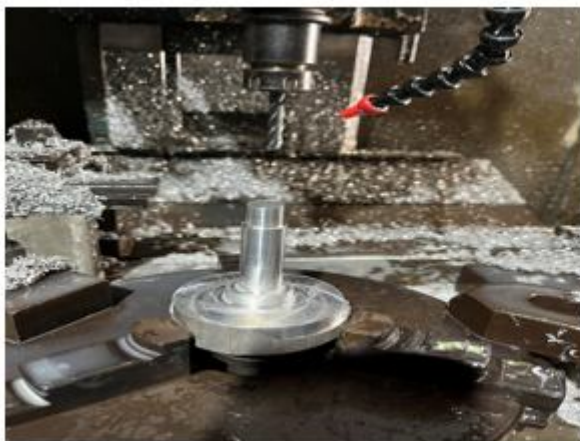
Figure 4 modified component manufactured and Tool bit used for process in CNC using Al 6061
