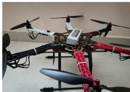
Figure. Assembled Drone
