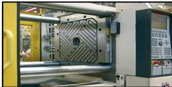
Fig 5:Quick mold changing system representation
