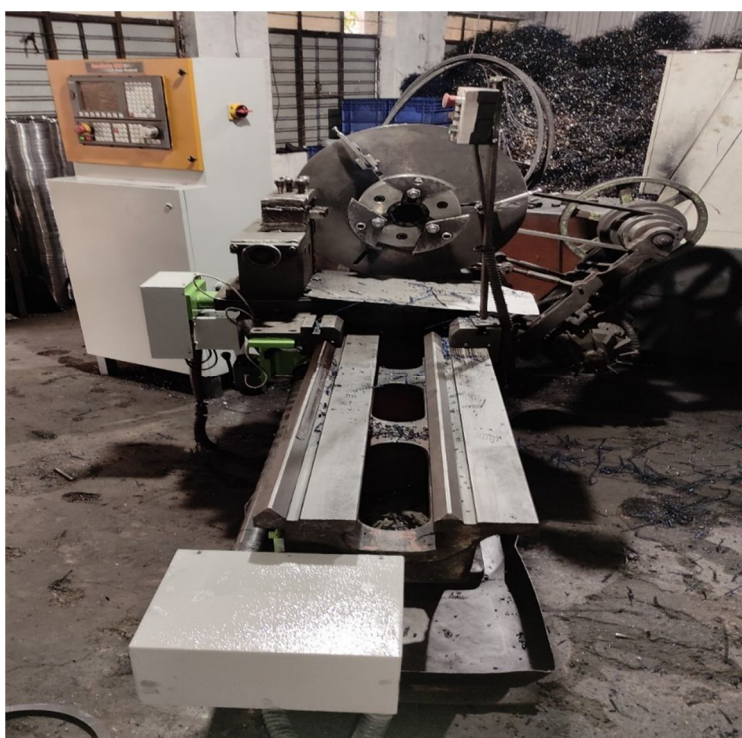
Fig. Lathe Bed of Modified Lathe Machine
