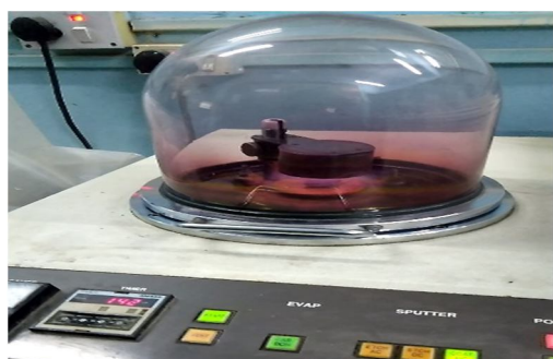
Figure 4: Gold Sputter coating machine
