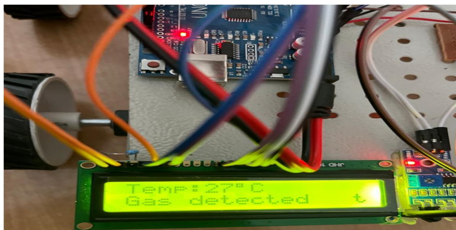
Figure 6 Robot displaying gas detection
