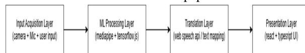
Fig. 1. Four-layer architecture of the MMACS platform illustrating data flow from hardware input through local ML inference to voice and text output.
