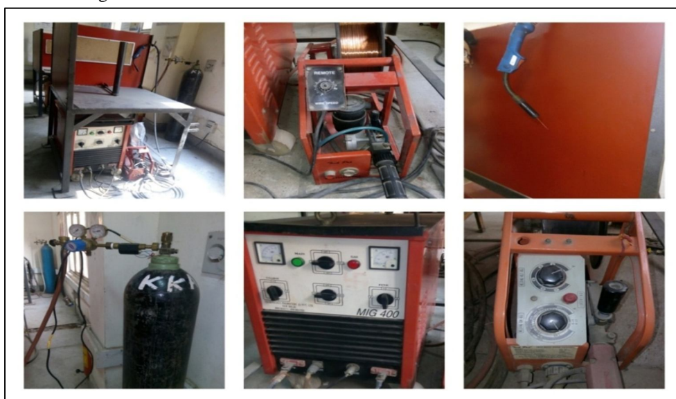
Figure 4: Different part of MIG welding setup
