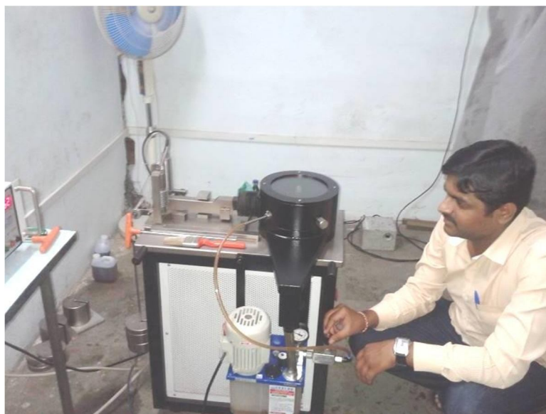
Fig. 9 Test Setup “Pin on Disk Tribometer”
