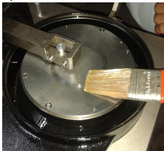
Fig. 8 Pin on Disk Tribometer including disk & pin.
