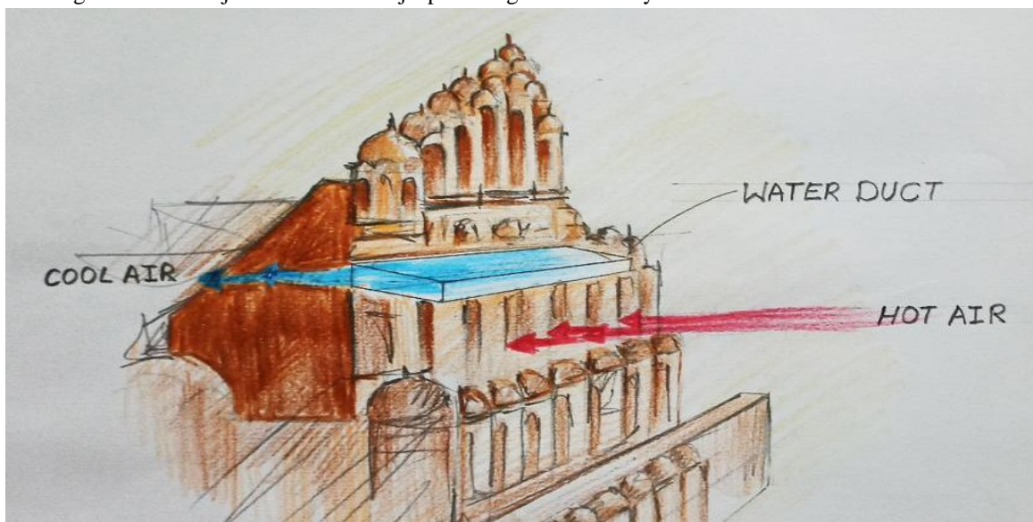
Figure 11: Wind movement through water ducts
