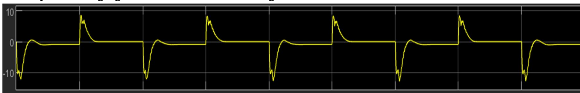
Fig 7 Ringing effect during switching
