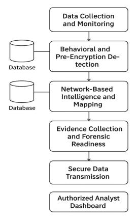
Figure-5.1: Data Flow Diagram (Dfd) For Netraptor
