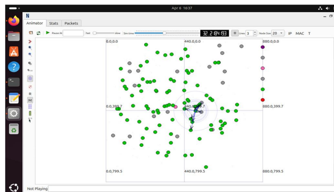
Fig. 11. NetAnim t = 32 s: LoRa CH elected; 92/92 users reconnected.
