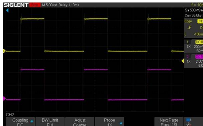
Fig.12. Gate signals of S1 and S2
