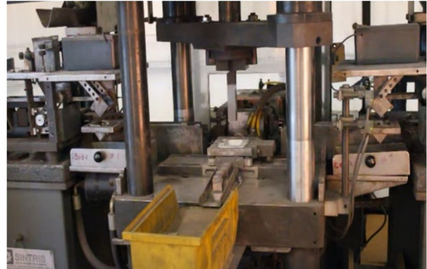
Fig 6 shows: Manufacturing of diamond tool blade
