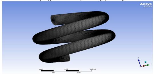
Upon completion of meshing, the annotation mesh components for the simulation analysis are performed by creation name selection for appropriate faces. The faces annotated as cold inlet cold fluid, outlet cold fluid, inner cold wall comprising of grooved area, and inlet hot fluid, outlet hot fluid, hot fluid wall.
