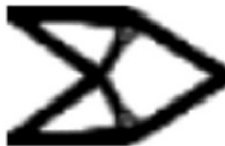
Fig. 4(b) Optimal layout using 1617 control points
