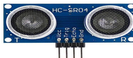
Fig 3.2: HC-SR04 Ultrasonic Sensor
