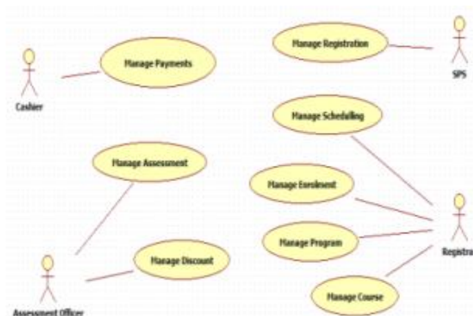
Fig. 1: Use Case Diagram
