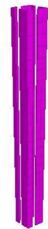
Fig. 8: Single Core Shear wall with 25 % opening and I = 1.5 (highest importance factor)
