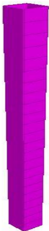
Fig. 4: Single Core Shear wall with 0 % opening and I = 1.5 (highest importance factor)
