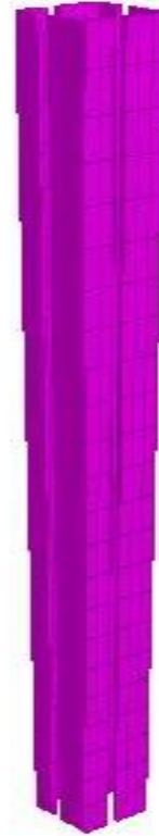
Fig. 7: Single Core Shear wall with 16.66 % opening and I = 1.5 (highest importance factor)
