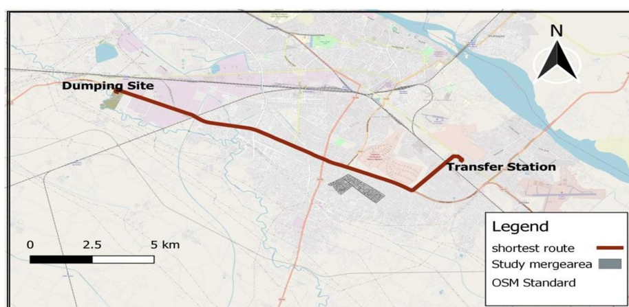
Fig:- 9 Shortest optimized solid waste collection vehicle route
