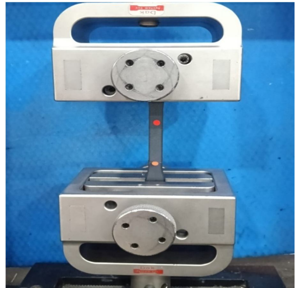
Figure 3: UTM setup used for tensile testing
