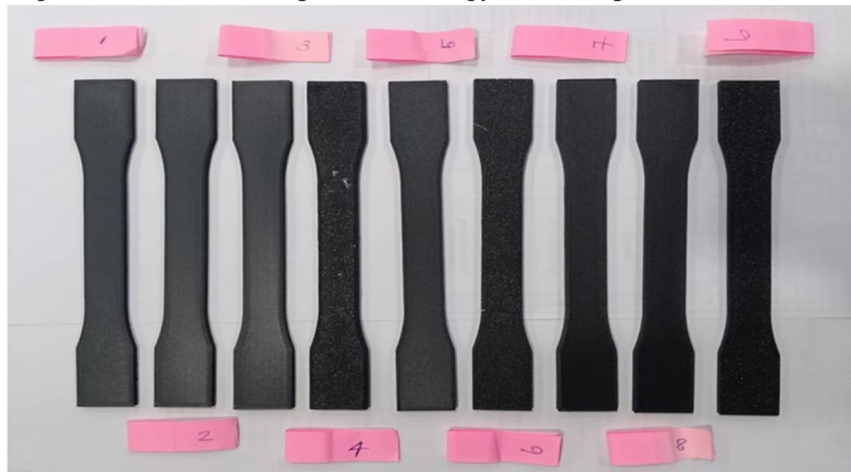
Figure 1: printed specimen according to ASTM D638 standard
