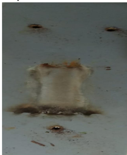
Fig 5.1 sample after 100 hours IPTE test
