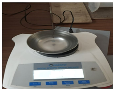
Fig 3.14: digital specific gravity balance meter
