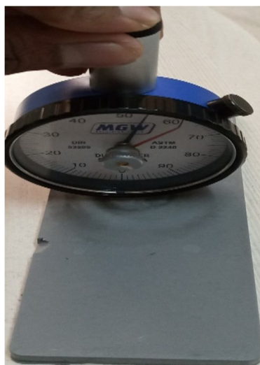
Fig 3.4: hardness measurement of polymeric test sample
