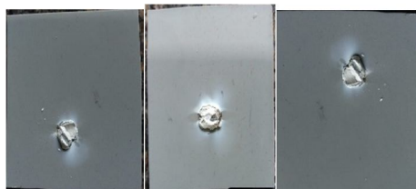
Fig 4.12: samples after the dry arc resistance test
