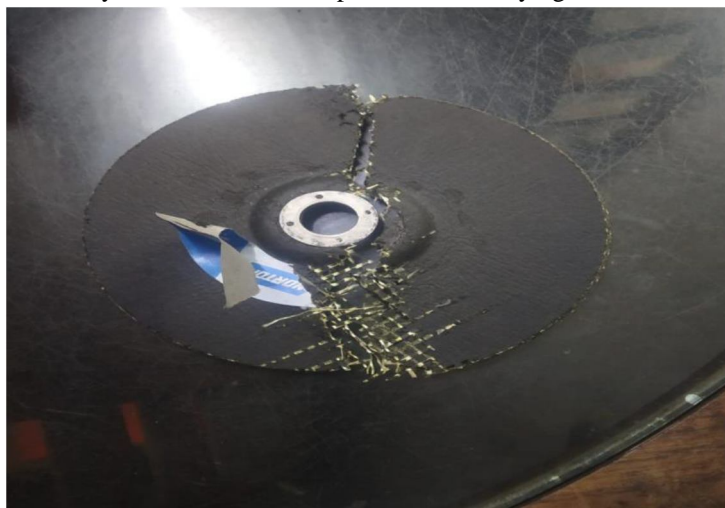
Fig Damage wheel while working
