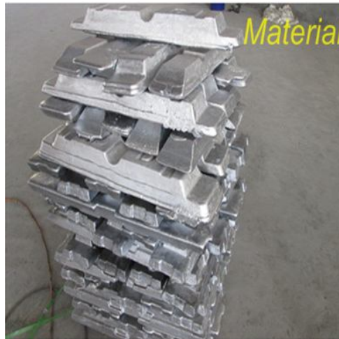
Figure 1.2: Aluminium material for die casting. [8]
