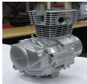
Figure 1.1: Aluminium die casted Automobile component having fins.
