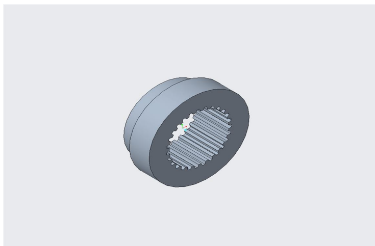
Fig 2.22 3d Model of Go Gauge
