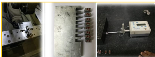
Figure 3.1: M/c Setup, work-piece and Ra measurement system
