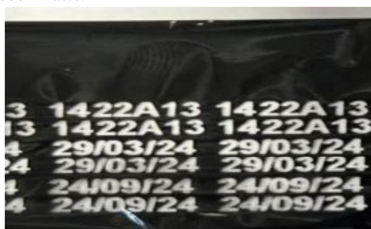
Fig. 5.2 Letter Height 2mm with Two Stagger Print
