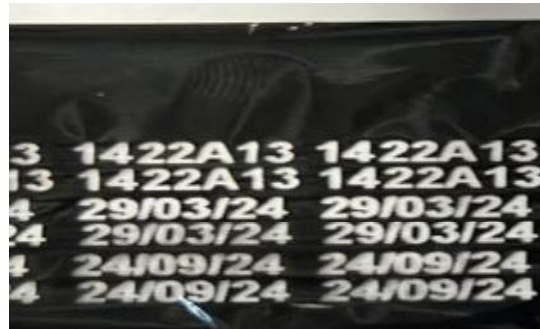
Fig. 5.2 Letter Height 2mm with Two Stagger Print
