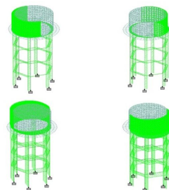
Fig 3. Wind loads acting on a tank
