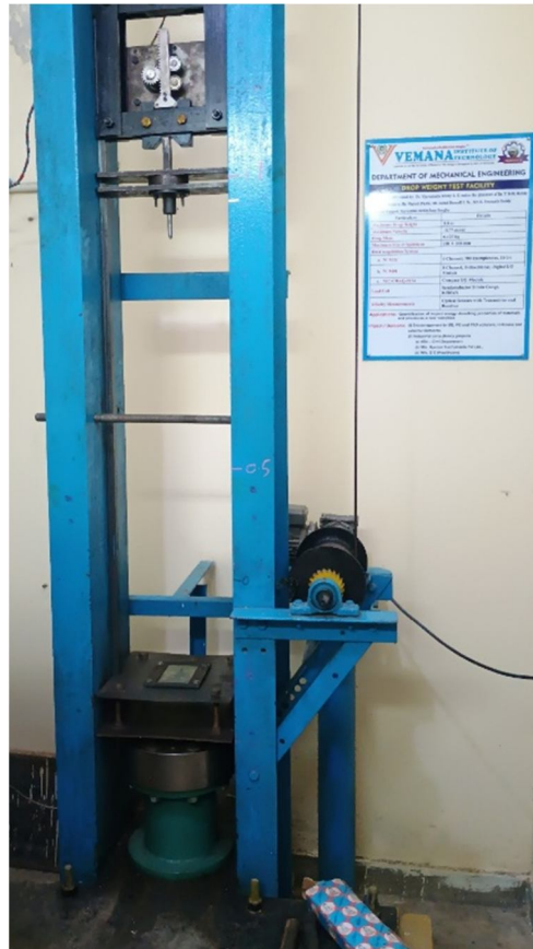
Fig 5. Drop weight impact test facility
