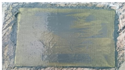
Fig. 1 The specimen after hand layup process
