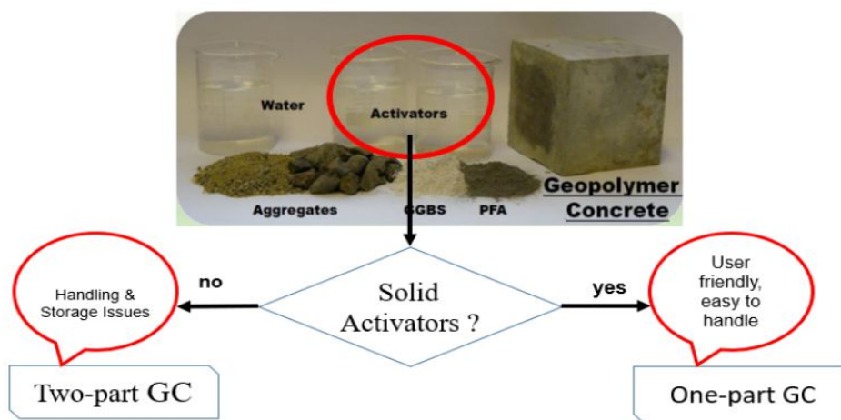
Fig. 3: Two-part & One-part Geopolymer Concrete
