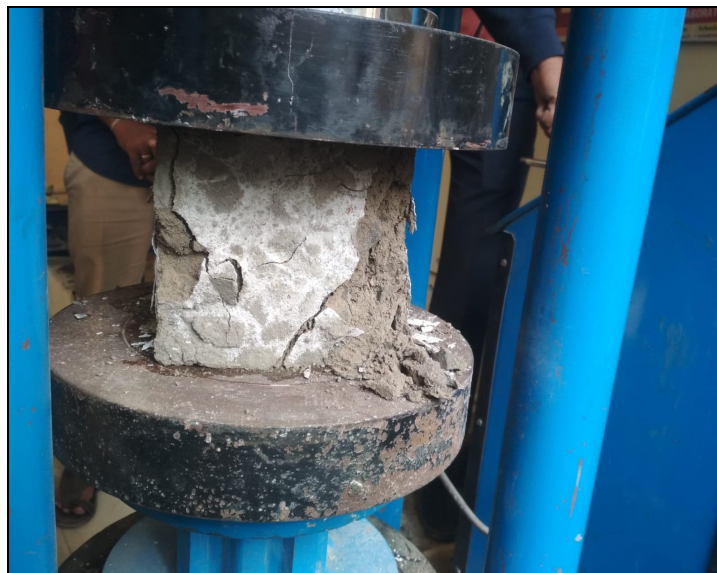
Fig. 7: (c) Testing of Geopolymer Concrete Cube under CTM
