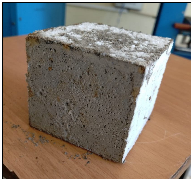
Fig. 6: (b) Demolding of Geopolymer Concrete Cube
