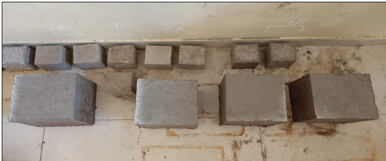
Fig. 5: (a) Casting of One-Part Geopolymer Cubes
