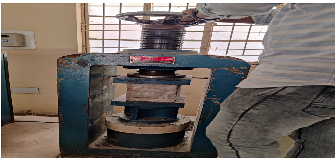
Fig. 4 Compressive strength test of cube
