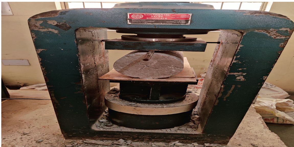
Fig. 2 Compressive strength of cylinder
