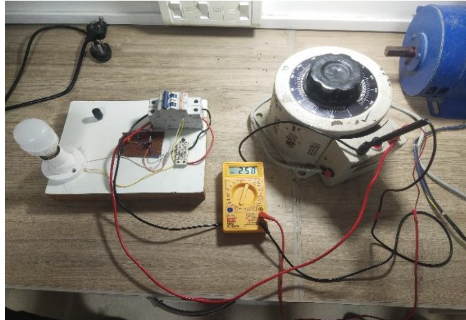
Fig .b) 3. Proposed system when there is an over voltage AC supply main.
